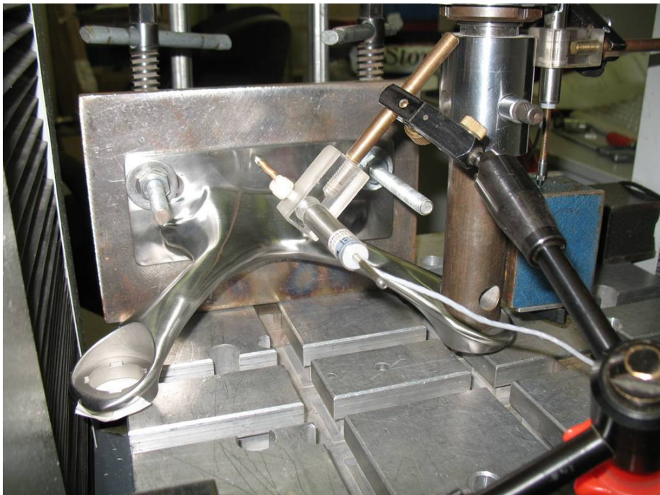
Perpendicular loading apparatus, determination of the permissible strength under instantaneous horizontal loads due to the wind on a 2-branch spider.
