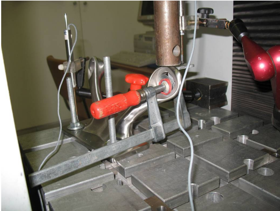
Parallel loading apparatus, determination of the permissible strength under permanent vertical loads (static load), on a 2-branch spider
